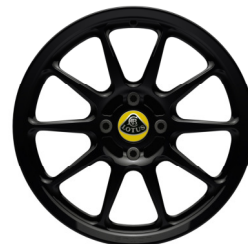
Gloss Black, 10-Spoke, Ultra lightweight 16" Front / 17" Rear, Forged
