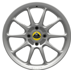
Optional Silver, 10-Spoke, Ultra lightweight 16" Front / 17" Rear, Forged
